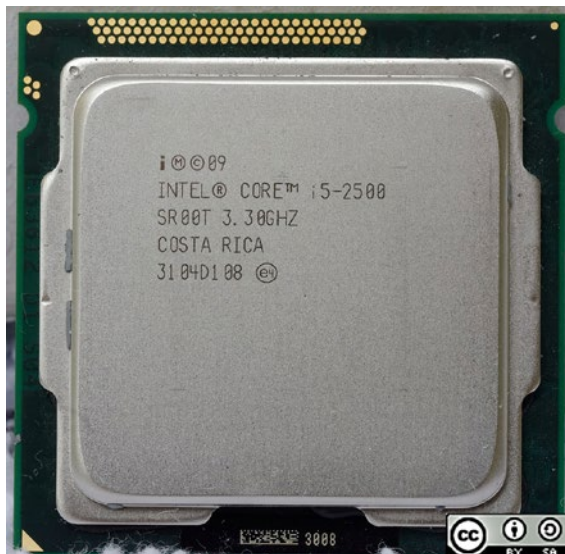
Figure 2-2. An Intel Core i5 processor may contain one, two, or four cores. Wikimedia Commons, CC by SA 4 International
