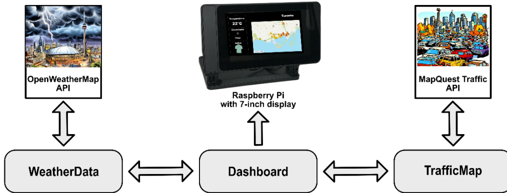
Figure 4.4 – Software architecture for the IoT information display
