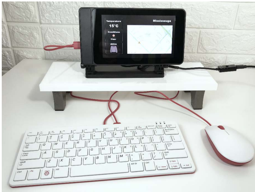
Figure 4.3 – Raspberry Pi development environment using a 7-inch touchscreen
