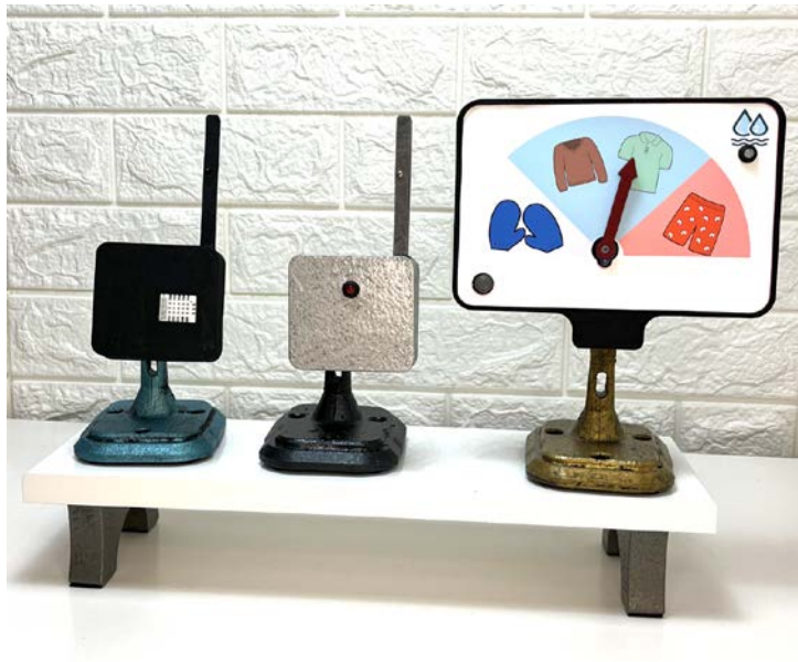
Figure 10.18 – The three devices that make up our IoT weather service, starting from the left, are the LoRa sensory transmitter ( Chapter 9 ), the LoRa receiver/ internet gateway ( Chapter 9 ), and the analog-metered weather indicator
