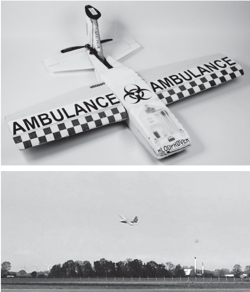
Figure 2.1 The prototype Danish healthcare drone developed to deliver urgent blood samples from outlying areas to major hospitals for analysis (top). The color scheme is modeled after a Danish ambulance; the drone is neon yellow with a dark green checker pattern on the leading edges of the wings, and the text is in red. The prototype Danish healthcare drone in context during testing at the Hans Christian Andersen Airport (bottom).
